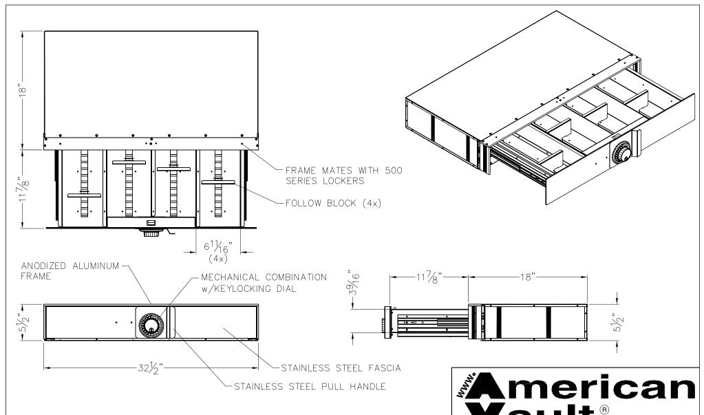
LOCKABLE FOUR COMPARTMENT CASH DRAWER WITH STAINLESS STEEL FASCIA AND ANODIZED ALUMINUM FRAME. FULLY ADJUSTABLE FOLLOW BLOCKS WITH POSITIVE LATCHING. FRAME MEMBER MATES WITH 500 SERIES LOCKERS.
