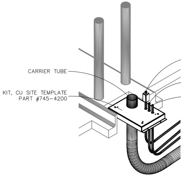
HOLD TEMPLATE LEVEL WITH TOP OF CONCRETE
